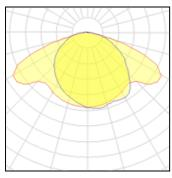
1 x Metal halide lamp Nominal lamp power 70 W LOR Lamp flux 7200 lm Total flux Luminous efficacy 62 lm/W Total power CCT 3000 K CRI 90
