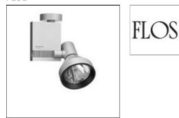
Range of indoor spotlights for accent and general lighting for three-phase track and wall/ceiling installation. Die-cast aluminium alloy, powdercoated optics compartment, diameter 118 mm, composed of an aluminium dissipating element placed above the lamp support, a black thermoplastic screen support ring and 4 mm tempered glass cover. Integrated auxiliary power units for the lamps inside a die-cast aluminium alloy container with powder-coated finish.
