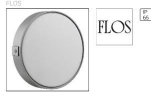
Guidelight designed for compact fluorescent lamps. Highly resistant injection-molded polycarbonate body. Highly corrosionresistant, die-cast aluminum front frame. Polycarbonate diffuser with or without die-cast aluminum anti-vandalism screen. Polyester powder-coated. Silicone gasket seals. Stainless steel screws. PG9 cable gland. Polycarbonate lamp support and reflector. Finishes: matt white (01), grey (72), matt black (04) and dark brown (MM).
