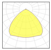
1 x High pressure mercury vapour lamp Nominal lamp power Lamp flux 24000 lm Luminous efficacy 47 lm/W CCT CRI
