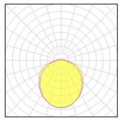
Lamp type LED CCT 4000 K 7.5 W CRI 80 Nominal lamp power Total flux 870 lm LOR 100% Luminous efficacy 116 lm/W ULOR 6% Total power 7.5 W
