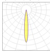
Lamp type Nominal lamp power Total flux Luminous efficacy LED 36 W 1720 lm 48 lm/W CCT
