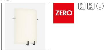
Finish: Dark-grey painted steel. Shade in matt opal glass. LED info: System power: 8W. Luminaire Luminous Flux: 590LM. CCT 3000K. SDCM 3. CRI 80. Installation: Wall installation. Connection: Snap-in terminal block 5x4mm2. Two cable entries. Design: Per Sundstedt.
