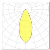
1 x Metal halide lamp Nominal lamp power 400 W LOR 80% Lamp flux 34000 lm Total flux 27288 lm Luminous efficacy 63 lm/W Total power 435 W CCT 5300 K CRI 90
