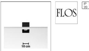
Desing for very low voltage lamps, discharge, main voltage and flourescent lamps. Pressed steel and matt black, powder-coated recessed housing, extruded aluminium recessed trim frame for use with false ceiling systems.
