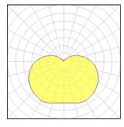
1 x Metal halide lamp Nominal lamp power 100 W LOR 59% Lamp flux 10000 lm ULOR 14% 51 lm/W Luminous efficacy Total flux 5889 lm 115 W CCT 3000 K Total power CRI 90
