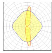
LED CCT 6000 K Lamp type Nominal lamp power 2.3 W CRI Total flux 100% 12 lm LOR Luminous efficacy 5 lm/W ULOR Total power 2.3 W
