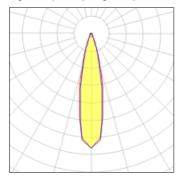
LED CCT 3000 K Lamp type Nominal lamp power 6 W CRI 80 Total flux LOR 100% 557 lm Luminous efficacy 93 lm/W Total power 6 W
