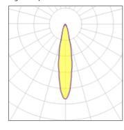
1 x LED Nominal lamp power Lamp flux 700 lm Luminous efficacy 54 lm/W CCT 3000 K CRI
