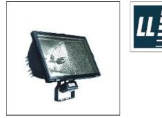
Small spots with halogen or high-pressure lamps for floodlighting historic/public buildings, open air/building sites, small sports fields, etc. -High-quality aluminium cast housing - Socket for halogen lamps with RSC-15 - Reflectors made of highest-grade aluminium sheet, burnished and anodized - Thermal protective glass - Silicone rubber seal - Special steel closing clips - Galvanized steel mounting bracket - Housing and bracket painted, see table for colours
