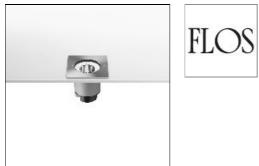
Adjustable recessed luminaire for ceilings or in ground applications, for LEDs or 12 volt halogen QR-CBC 35 lamps. Die-cast aluminum recessed housing, high corrosionresistance. 6mm tempered protection glass. Silicone seals. Stainless steel closing ring with fixing screws. PG9 cable gland with pre-wired 1 metre power loom. Finishes: matt black (04), grey (72), stainless steel (55), stainless steel dark copper (PB), stainless steel gold (PG), stainless steel black (PN).
