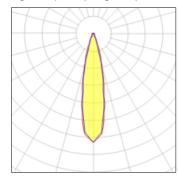
LED CCT 2700 K Lamp type Nominal lamp power 6 W CRI 80 Total flux LOR 100% 528 lm Luminous efficacy 88 lm/W Total power 6 W
