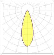
CCT Lamp type LED Nominal lamp power 26 W CRI Total flux 2500 lm LOR 96 lm/W Luminous efficacy Total power
