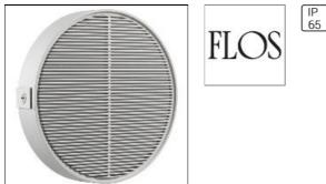
Guidelight designed for compact fluorescent lamps. Highly resistant injection-molded polycarbonate body. Highly corrosionresistant, die-cast aluminum front frame. Polycarbonate diffuser with or without die-cast aluminum anti-vandalism screen. Polyester powder-coated. Silicone gasket seals. Stainless steel screws. PG9 cable gland. Polycarbonate lamp support and reflector. Finishes: matt white (01), grey (72), matt black (04) and dark brown (MM).
