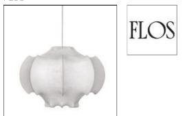
Suspension lamp providing diffused ligh-ting. White powder coated internal steel structure sprayed with a unique "cocoon" resin to create the diffuser which is then protected by a transparent sprayed on finish. Power cord length 4000 mm.Net weight 1,75 kg.
