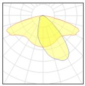
Lamp type LED Nominal lamp power 31 W Total flux 3628 lm Luminous efficacy 117 lm/W
