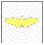
Lamp type LED Nominal lamp power 10 W Total flux 490 lm Luminous efficacy 49 lm/W
