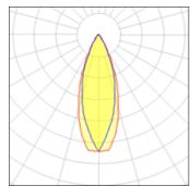
1 x Metal halide lamp Nominal lamp power 70 W Socket G8D.5 Lamp flux LOR 6900 lm Luminous efficacy 35 lm/W Total flux 2463 lm CCT 3000 K Total power 70 W CRI 83
