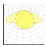
1 x High pressure mercury vapour lamp
