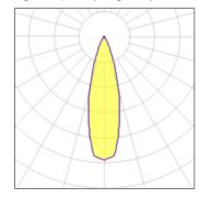
Lamp type LED CCT 4000 K Nominal lamp power 8 W CRI 80 Total flux LOR 100% 556 lm Luminous efficacy 70 lm/W Total power 8 W
