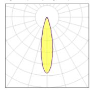
LED CCT 3000 K Lamp type Nominal lamp power 4 W CRI 80 Total flux LOR 100% 158 lm Luminous efficacy 40 lm/W Total power 4 W
