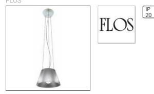
Suspension lamp providing diffused ligh-ting. Acid-etched pressed borosilicate glass internal diffuser. Pressed clear glass shade. Injectionmolded transparent poly-carbonate diffuser support. Transparent, stamped polycarbonate dust protection screen. White, injection-molded ABS rose, galva-nized pressed steel ceiling fitting. Steel suspension cables and polarized double-insulated PTFE cord, length 4000 mm. Net weight 4,5 kg.
