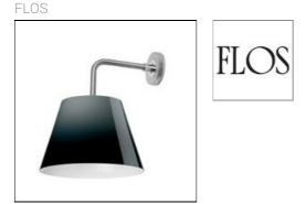
Wall or floor luminaires for outdoor use providing direct and diffused light. The outdoor range of luminaires has: a die-cast aluminum alloy wall or ceiling fitting with brillant finish; an injection-molded polycarbonate (PC) cover rose; a 316L stainless steel stem-polished; an opal-colored, vacuum-formed internal polycarbonate diffuser
