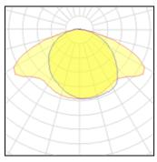
1 x Metal halide lamp Nominal lamp power 100 W LOR 78% 7797 lm Lamp flux 10000 lm Total flux Luminous efficacy 68 lm/W Total power 115 W CCT 3000 K CRI 90
