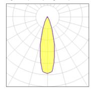
LED CCT 4000 K Lamp type Nominal lamp power 8 W CRI 80 Total flux LOR 100% 556 lm Luminous efficacy 70 lm/W Total power 8 W
