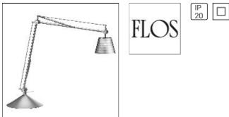
Task lamp providing direct and diffused light. Acid-etched pressed borosilicate glass internal diffuser. Injection-molded PC (polycarbonate) diffuser, vacuum-aluminized inside. Gray painted die-cast aluminum diffuser support. Gray painted assembly composed of extruded aluminum arms, steel tie rods, stainless steel springs, and 50% fiberglass reinforced, injection-molded polyamide joints. Gray painted die-cast Zamak BASE.
